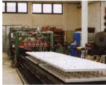
The EPS slabs are shaped from Expanded Polystyrene (EPS) beads through a process of expansion, conditioning and molding, post processing, and cutting to EPS slabs of desired density. Production process of the EPS slabs permits consistently high quality of eWall modules to be achieved with distinct material, time, cost, and lightweight benefits.
